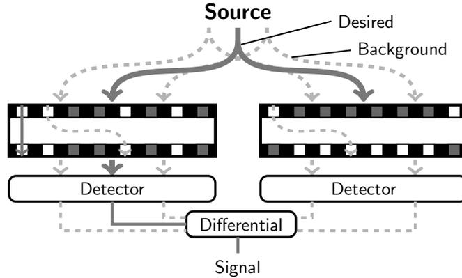
Figure 1: Golay's spectrometer design
